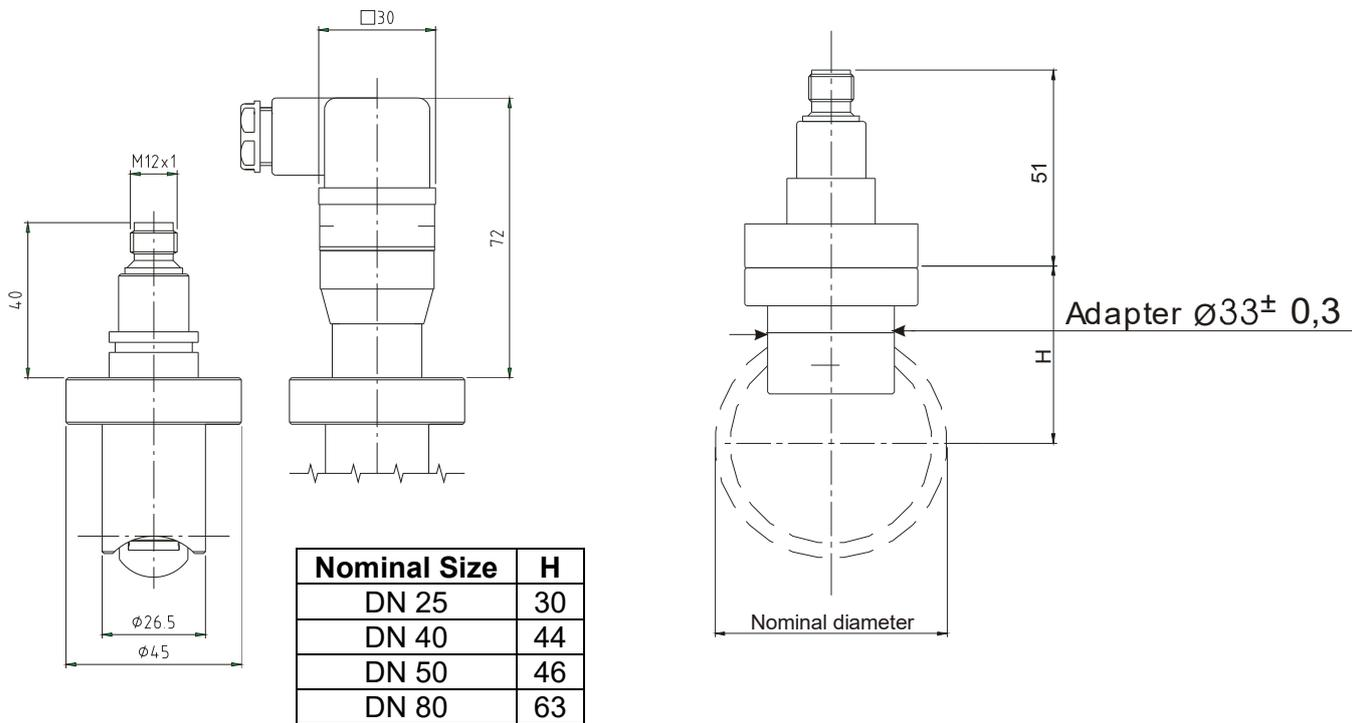
Position and weld-in the mounting adapter according to the nominal diameter suitable marking. The marking on the adapter must be in line with the outer diameter of the pipe. Also pay attention to the later position of the rotating vane (shaft of the vane shifted by  $90^\circ$  to the direction of flow).
