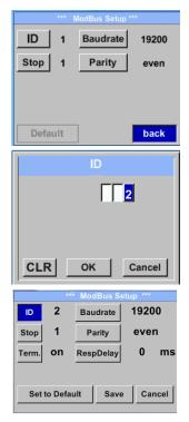
For changes, e.g. the sensor ID, first select by pressing key "△" the field "ID" and then key "OK".
