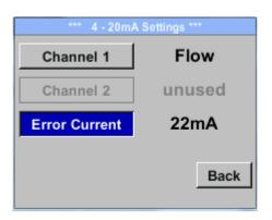
This determines what is output in case of an error at the analog output.
