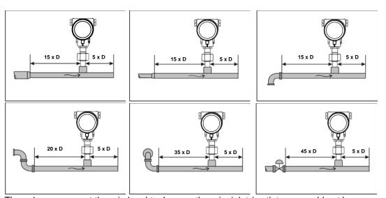
The values represent the min.lenghts. In case the min. inlet / outlet runs could not be ensured, it must be expected to get increased or significant d eviations of the measurement values.
