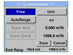
The 4-20 mA Analogue output of the Sensor KEC can be individually adjusted.
