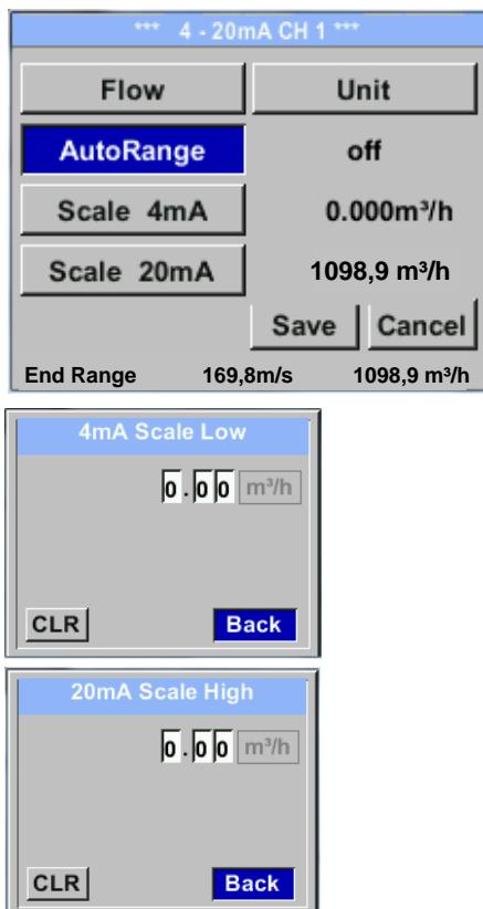
The scaling of the 4-20mA channel can be done automatically "Auto Range = on" or manual "AutoRange = off".
