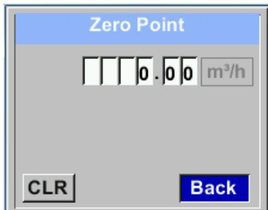
When, without flow, the installed sensor shows already a flow value of > 0 m³/h herewith the zero point of the characteristic could be reset.
