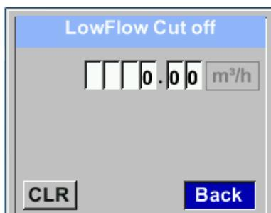
With the low-flow cut off activated, the flow below the defined "LowFlow Cut off" value will be displayed as 0 m³/h and not added to the consumption counter.
