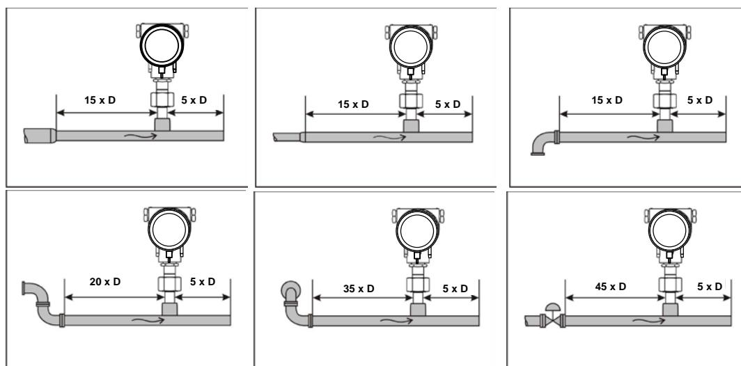
The values represent the min. lengths. In case the min. inlet / outlet runs could not be ensured, it must be expected to get increased or significant deviations of the measurement values.
