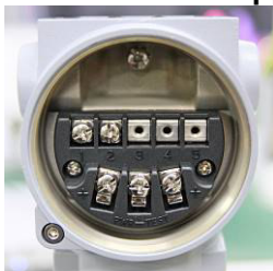
1: Pulse Output+, 2: Pulse Output-
