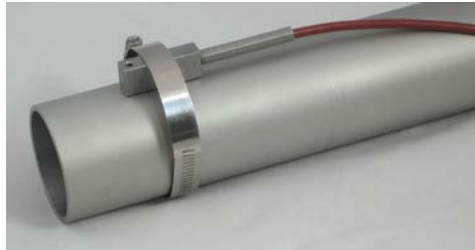
Figure 22: At pipe mounted Pt100
