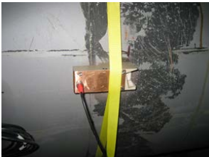
Figure 33: Textile tension bands are recommended for the assembly of the DUC-WP05 transducers (temperature limitation)
