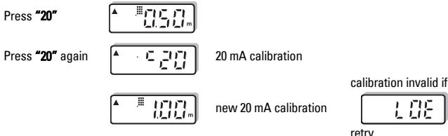
**Note:** Calibration bypasses the measurement response rate.
