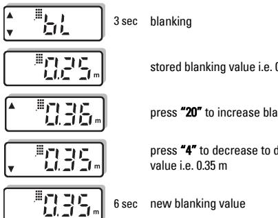
**Note:** For faster scrolling, hold the key depressed during the blanking adjustment and release when desired value is obtained.
