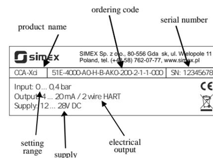
Fig. 1 manufacturing label- example
