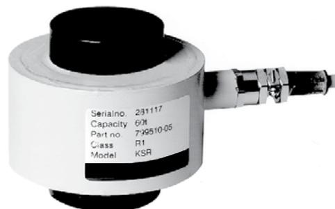
A reliable sealing and mechanical protection of the strain gage area is ensured by the use of stainless steel diaphragms and an epoxy coated alloy steel housing, both of which are cemented to the measuring element.
