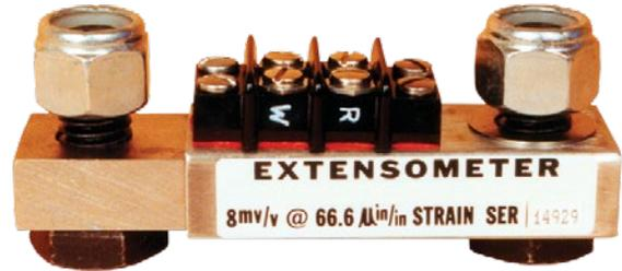
With extensometers installed, the mill posts become an active part of the measuring system. The entire mill housing with the attached extensometer can be considered a "load cell".
