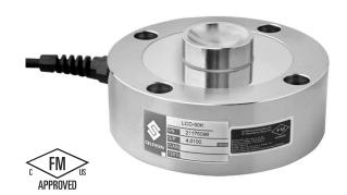
The low profile compression disk is designed as the ultimate solution for some difficult applications in which height is a major safety concern. The shear web design provides excellent performance even when side force inevitably exists in normal operations. A typical example of such side force can be found in motor truck scales, making the model LCD perfect for such applications.
