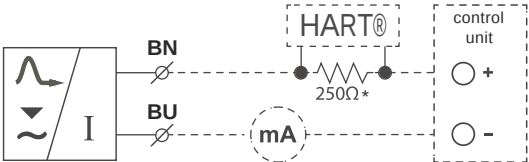
Connection diagram of the level gauge with current output CPC-AR-54
